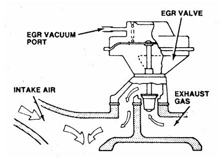
Advanced methods use solenoids to open and close the EGR valve. The solenoids are toggled by signals from the microprocessor which acts accordingly to signals received from various sensors on the engine. The electronically managed EGR valves operate more precisely than the vacuum managed valves and they are also more expensive. Therefore before you condemn the EGR valve, perform an analysis to verify the EGR is receiving the signals. If not, a new one won't be of any help.
