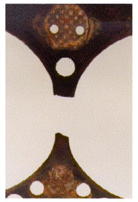
We do want to point out that a defective EGR valve is not the Lone Ranger in destroying head gaskets. It's only one of the causes but one of the most common. The ignition timing, clamp load and surface finish are equally as important. And, last but not least, is the entire cooling system.
