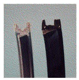
This design also works for one-piece seals, although it requires more engineering analysis. In the case of the one-piece seal, the engine builder could chose between using a repair sleeve or the offset lip. We suggest the use of the seal first, since this will allow you to have a core that can be used with a repair sleeve the next time around.
