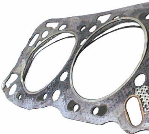
Radial splitting of bore ferrules
