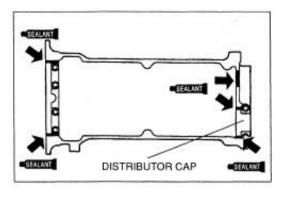
The use of a good quality sensor safe sealant such as ThreeBond TB004 is recommended. Apply to areas as required (see illustration as a guide) and allow 7 - 10 minutes for the sealant to surface dry then fit parts immediately. Tighten cover to specified torque.
