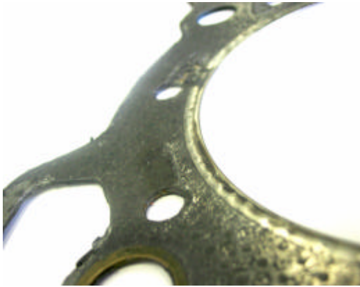
Radial indentation damage to bore ferrules
