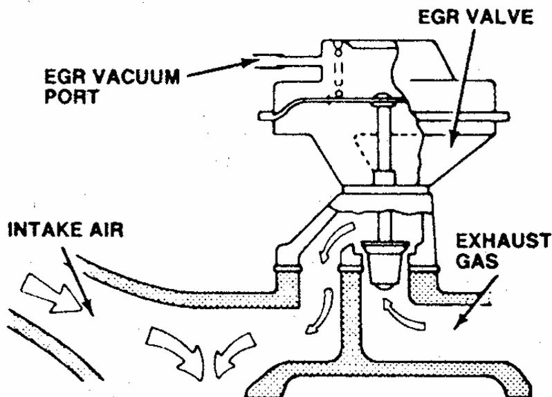
Advanced methods use solenoids to open and close the EGR valve. The solenoids are toggled by signals from the microprocessor which acts accordingly to signals received from various sensors on the engine. The electronically managed EGR valves operate more precisely than the vacuum managed valves and they are also more expensive. Therefore before you condemn the EGR valve, perform an analysis to verify the EGR is receiving the signals. If not, a new one won't be of any help.
