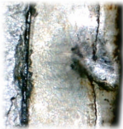
Trapped debris damages gaskets fire-ring
