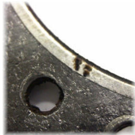
Debris can allow leak paths for combustion
